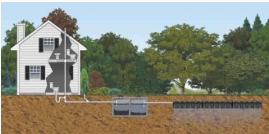
A conventional soil absorption system is expected to last a minimum of 30 years if properly designed and maintained.
