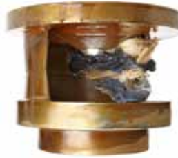
Figure 4: Accumulation in a single-vane impeller
