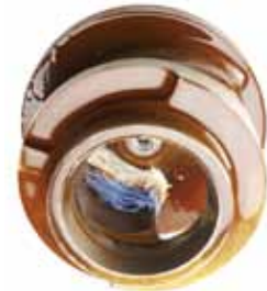
Figure 5: Accumulation in a single-vane impeller
