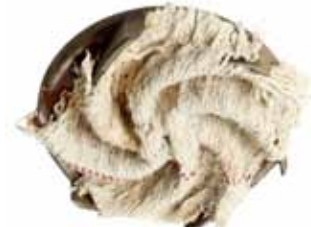
Figure 7: Accumulation in a vortex impeller
