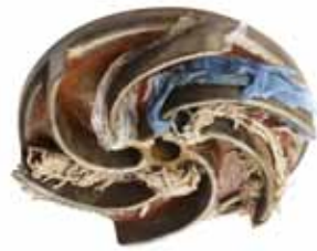
Figure 6: Accumulation in a vortex impeller
