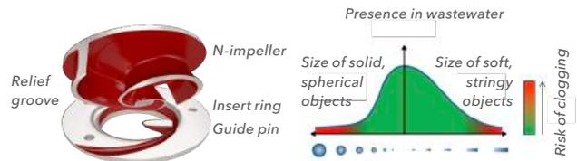
Figure 6: Self-cleaning pump - Hydraulic part
