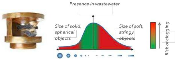
Figure 4: Clogging in channel impellers
