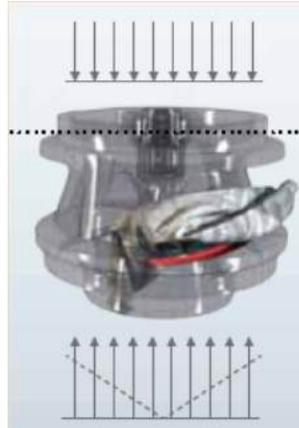
Figure 11: Force distribution when debris enters the pump
