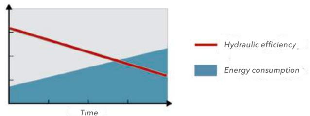
Figure 13a: Traditional pump running continuously
