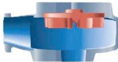
Figure 2: Vortex impeller
