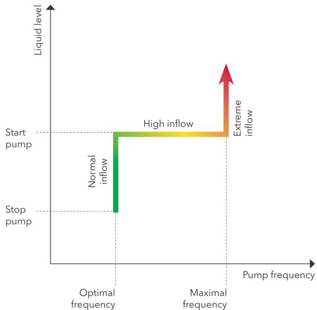
Figure 12: Optimal constant level control.
